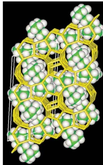
*Location of structure-directing cations in the pores of zeolitic material CIT-1, as determined in ref. [7]. This model was found to be the only possible fit to both data and theory. This determination required multiple rounds of experimental*
